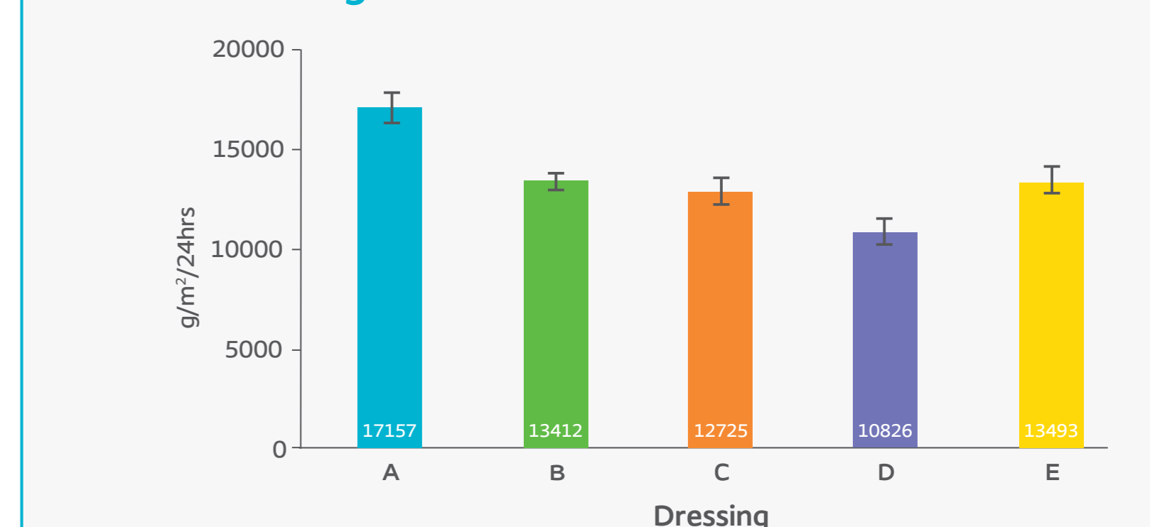
Figure 7: The average fluid handling capacity of five dressings*. The fluid handling capacity is the summation of absorption and permeability. n = 10 .
